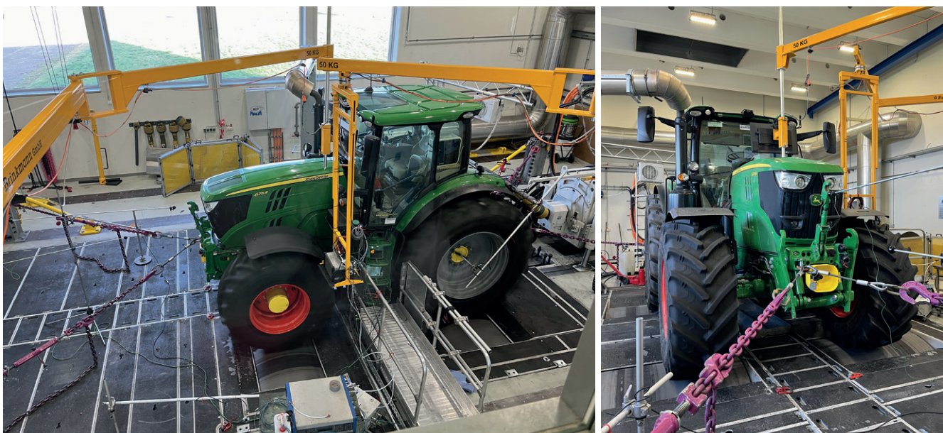
Figure 6: Transport run on the DLG chassis dynamometer
